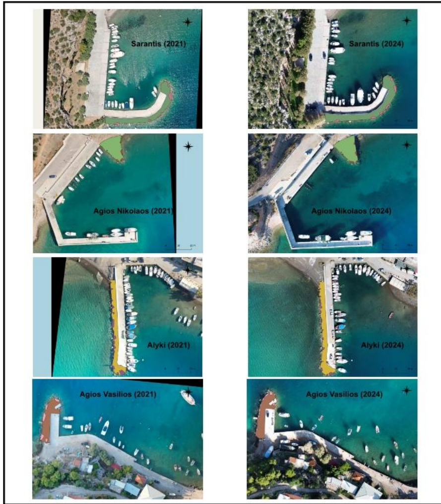
Figure 8. Port vulnerability changes regarding the parameter of armor layer displacement.
