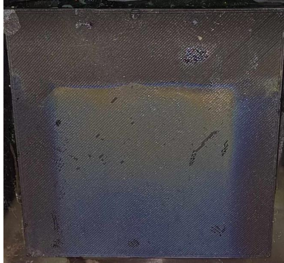
Figure 18: Cathode with the MnO_2 coating on the outer side
