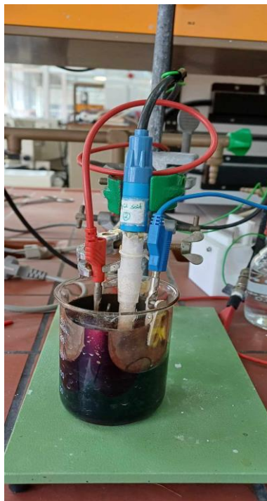
Figure 9: Experimental setup used for OCV, CV and Mn deposition
