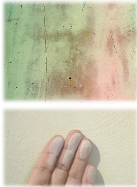
Figure 65: Chalking and its “powdery” feeling on hand (PST, Photo Gallery, 2015)
