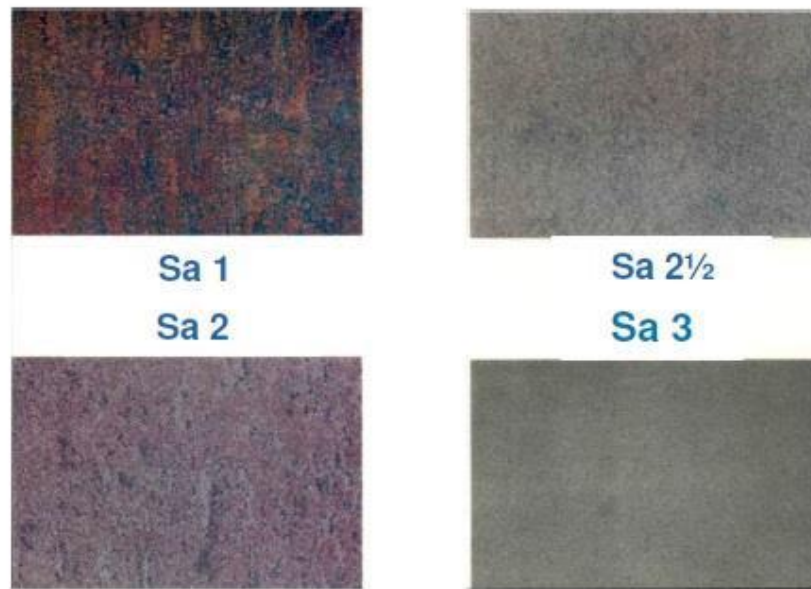
Figure 42: A sample of the norms Sa1, Sa 2 ½, Sa 2 and Sa 3 (PST, Photo Gallery, 2015)
