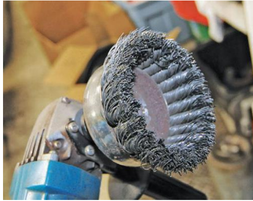
Figure 4: A wire-brush, one of the methods of dealing with rust, as mentioned above (PST Photo Gallery, 2015)
