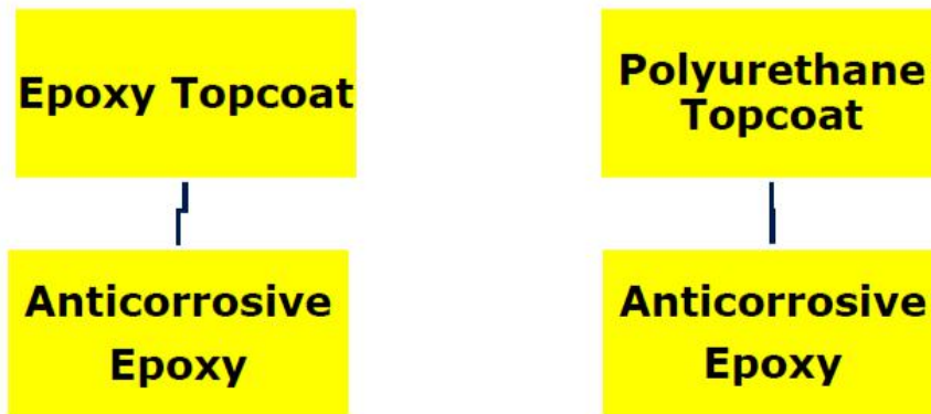
Figure 8: Paint systems (Compatibility of Generic Types) (2) (ABS Coating Performance Standards, 2019)
