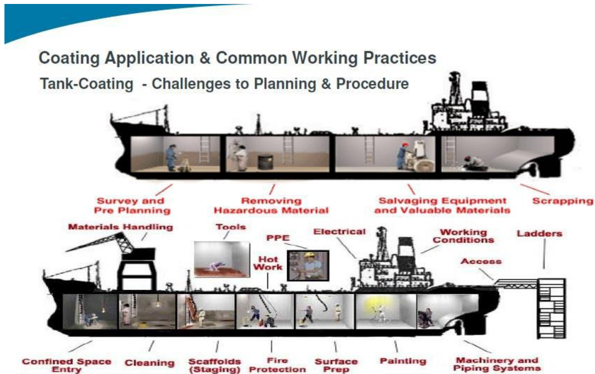
Figure 6: A diagram of the most important stages and factors affecting tank-coating (many of which will be examined furthermore afterwards) (Hyundai Painting Specification, 2016)
