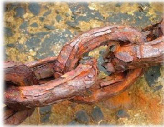
Figure 38: Part of the ship chain corroded (PST Photo Gallery, 2015)
