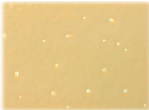
Figure 84: Fish eyes (1) (How to select the right paint system, Hempel, 2019)
