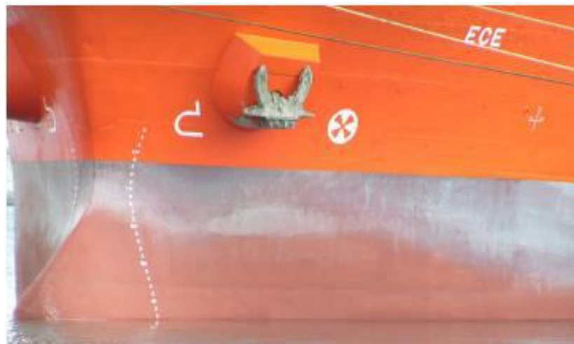
Figure 76: The blue-ish colour because of the reaction of the cuprous oxide with the components of the sea water (PST, Photo Gallery, 2015)
