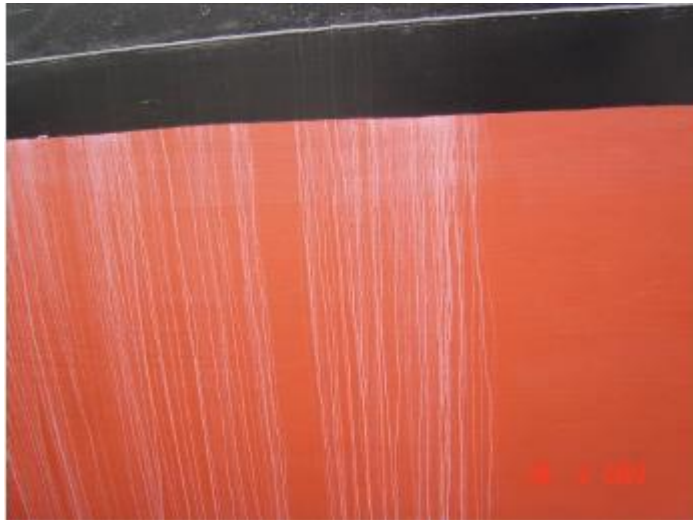
Figure 74: The whitening of anti-fouling coating due to premature water exposure (PST, Photo Gallery, 2015)
