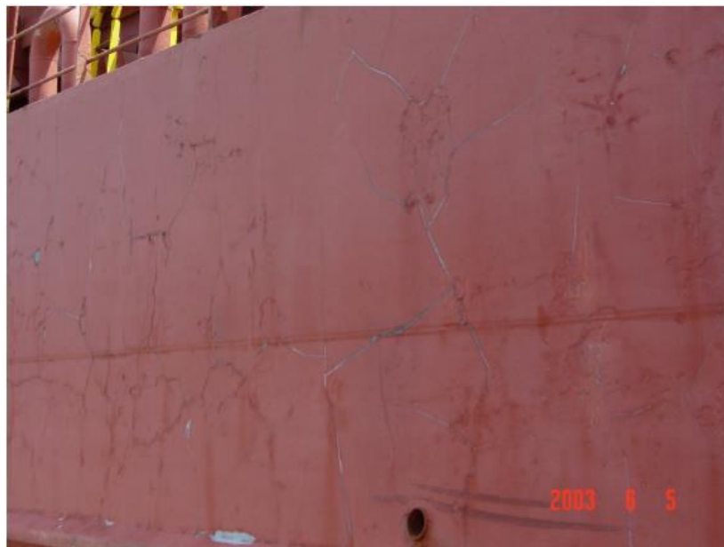
Figure 72: Cracking (5) (PST, Photo Gallery, 2015)
