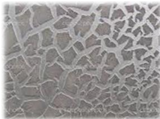
Figure 61: Alligatoring (Coating Manual, Jotun, 2018)
