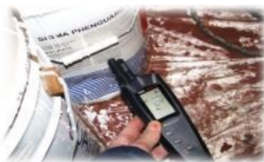
Figure 8.1.1: Measuring Dew Point with the help of PDS (PST, Photo Gallery, 2015)
