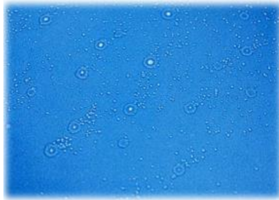
Figure 85: Fish eyes (2) (How to select the right paint system, Hempel, 2019)
