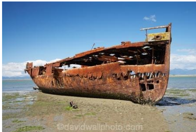
Figure 1: Extended levels of rust on a shipwreck, located in New Zealand, (Jotun Coating Manual, Athens, 2018)
