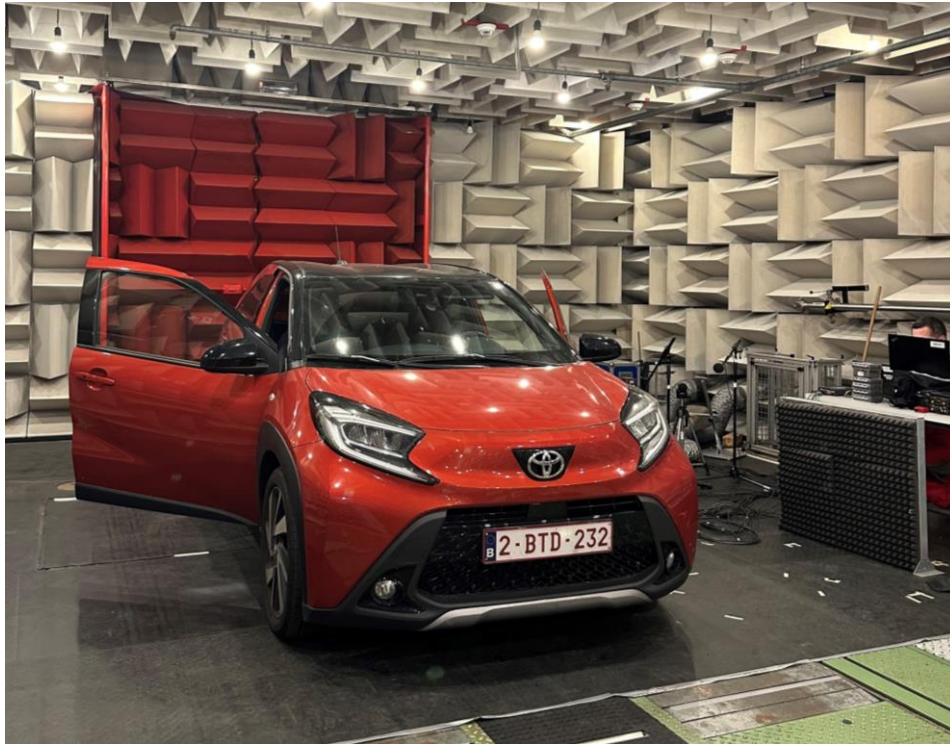
Figure 6.6-1: Placement of the vehicle inside the anechoic chamber to minimize the effect of unwanted environmental noise in the measurement.
