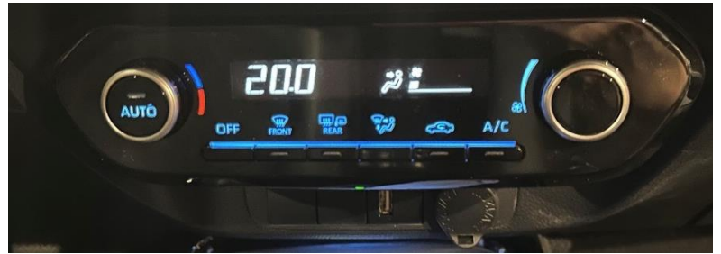
Figure 6.6-5: HVAC mode settings. Blower was set to face mode, temperature to 20°C and the flux to the respective scale from 1 to 7.
