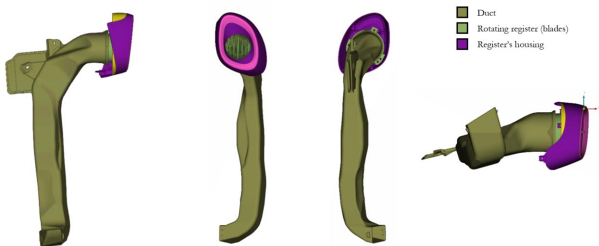
Figure 1.2-2: The blower assembly of side-duct of car 1 with its components.
