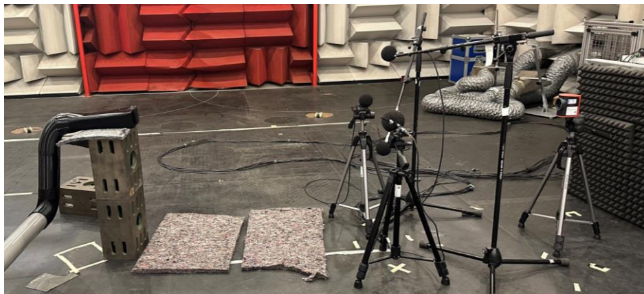
Figure 6.5-2: Microphone positioning for the measurement of background noise for all center duct configurations.
