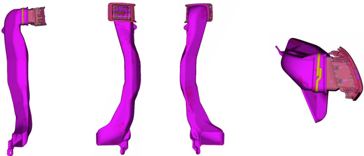
Figure 6.2-4: Side-duct assembly of car three.
