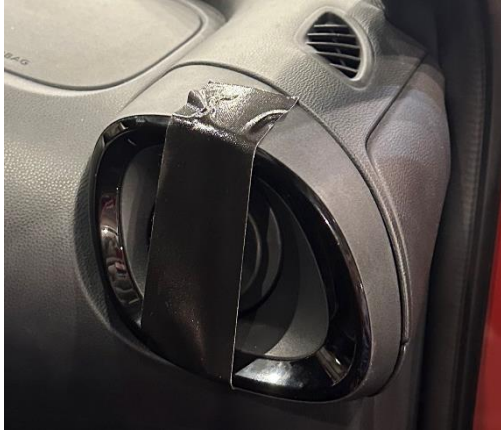
Figure 6.6-4: Sealing of the passenger – side blower to avoid impairing the results of the measurement. The duct tape put on the outer casing of the register is to visualize that it has been sealed.
