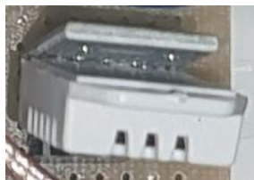
Figure 94 The DHT22 air humidity/temperature sensor which is used in order to have a sense of the conditions inside the device.
