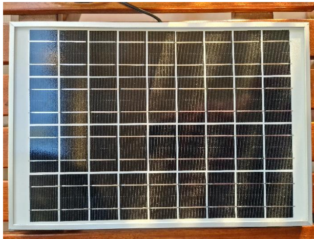
Figure 110 The solar panel used in order to supply with power the resin collection device.
