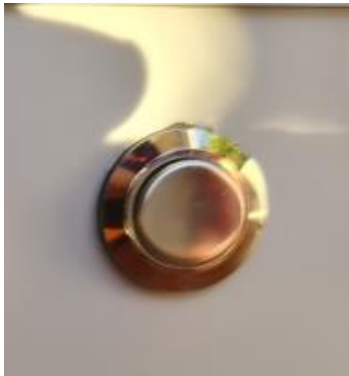
Figure 103 Push-button, that the user uses when they want to get information in the LCD screen instantly.
