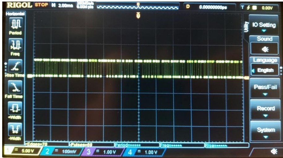
Figure 24 In the picture someone can see how is a signal (message) that is sent from the Arduino (existing in the basil pot) to the Raspberry Pi, via Xbee Zigbee is viewed under the oscilloscope. The current needed from the Xbee Zigbee module is around 40 mA, according the manufacturer 9 . The whole device operates at 5 Volts, which results in a power consumption of P = V * I = 5 * 40 \text{ mA} = 200 \text{ mW} on peak of the signal.
