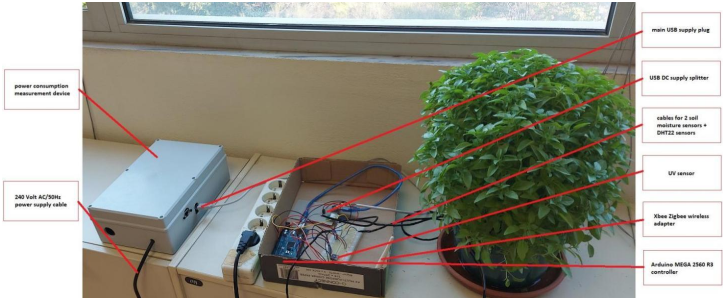
Figure 3 View of the infrastructure for sensing the parameters of the basil pot (temperature, humidity, UV radiance) and the measuring device, which measures and data-logs Voltage, Current and Power consumption.
