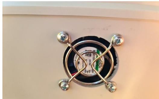
Figure 101 The fan responsible to cool the whole circuit and the battery when there is increased temperature inside the box.
