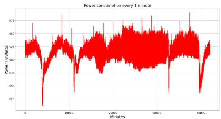
Figure 23 Power consumption of the completed circuit, measured in mWatts, with 1 minute sampling frequency.
