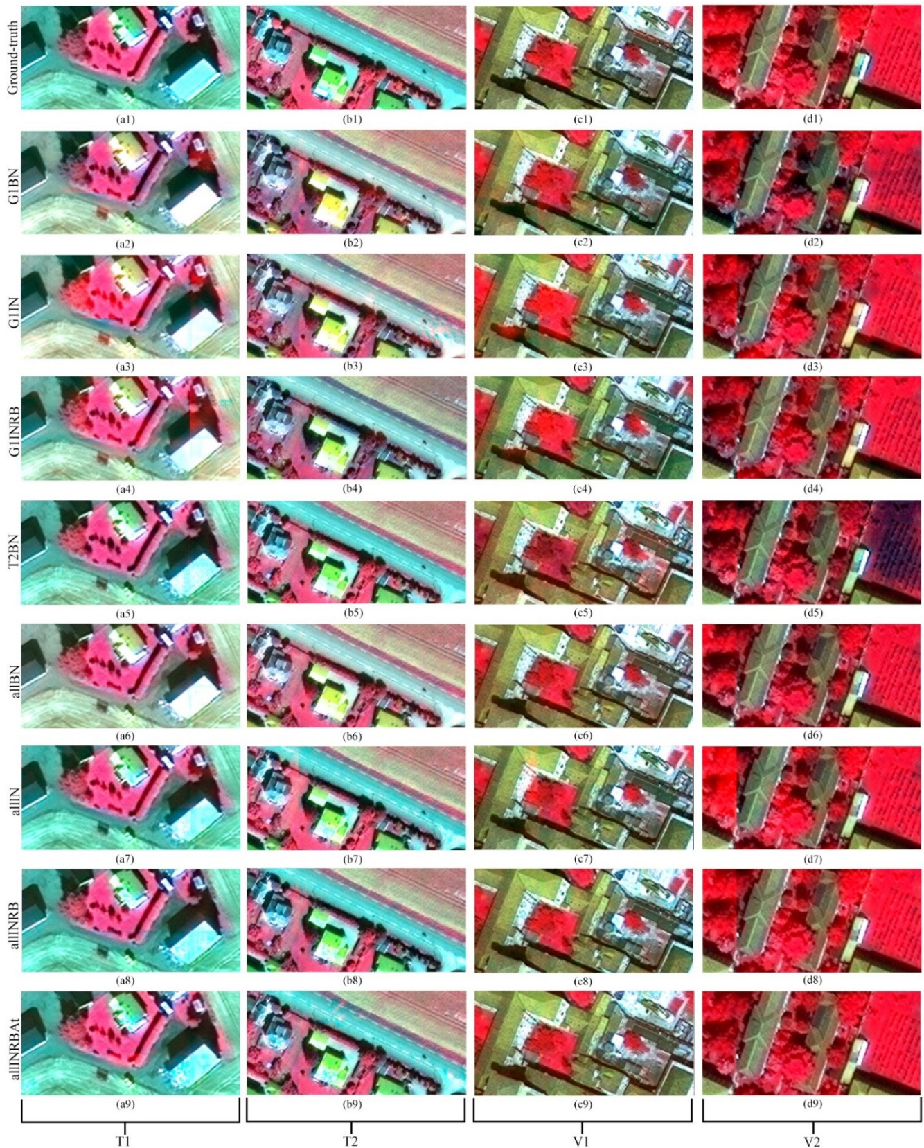
Figure 5.8. Samples of pseudo-color composites of the NIR predictions in the paired ITIT (Tønsberg, Venice) – first stage. Red color is assigned to the NIR band, green color to the RED band, and blue color to the GREEN band.
