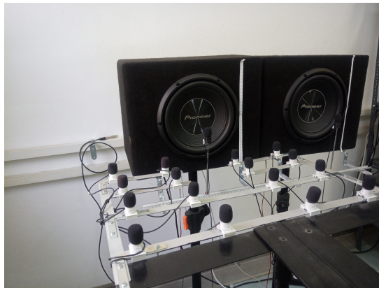
Figure D.1: The metallic grille, where 16 measurement microphones were mounted in order to monitor the acoustic pressure before and after the ANC activation.
