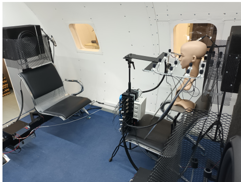
(a) Opposite local ANC systems in the small aircraft cabin mockup installed in the Dynamics and Acoustics Laboratory
