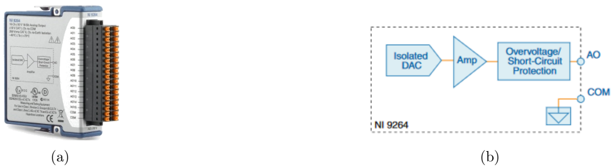
Figure C.4: a) Digital to analog converter (DAC) NI 9264, b) block diagram of NI9264 [148].
