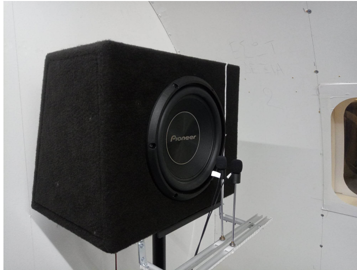
Figure 6.6: The active absorber based on sound wave separation method
