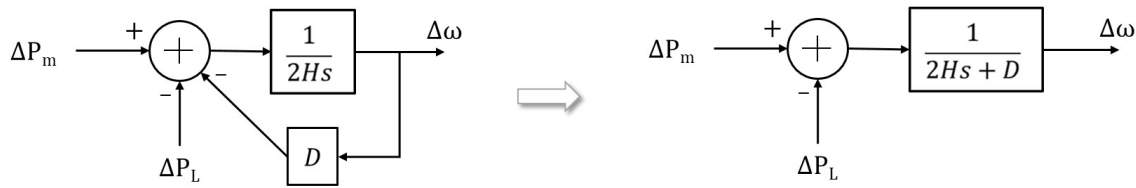
Figure 3.2 Generator transfer function considering load changes.
