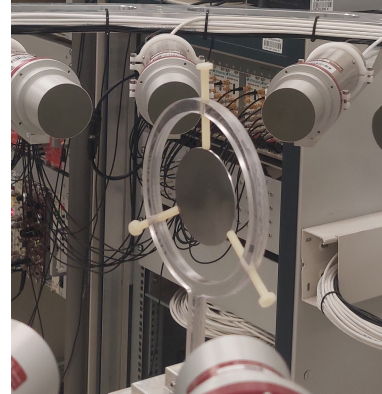
Figure 3.1: Photo of the ^{56}\text{Fe} sample placed in the sample position of the ELISA spectrometer.
