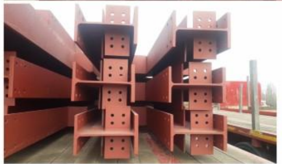
b) Reclaimed steel ready for the new use
