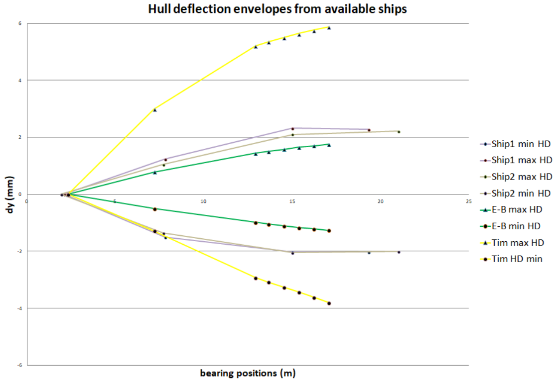
Figure 47: Calculated hull deflections envelope compared to available data
