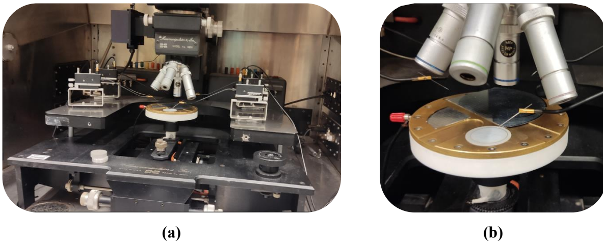
Figure 6.2 The probe station used for the electrical characterization of the samples
