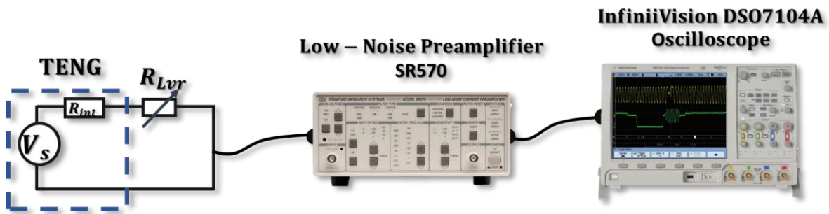
Figure 7.12 Schematic illustration to measure electrical currents generated by TENG device using SR570.
