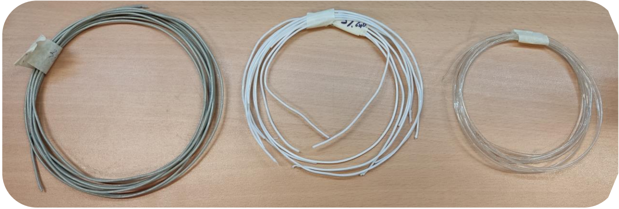
Figure 4.5 From left to right: PLA – 3wt% SiC, PLA – 3wt% ZnO, PLA virgin.
