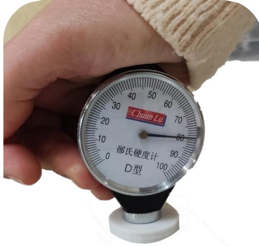
Figure 5.8 The Shore D durometer used for hardness measurement.
