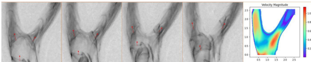
Figure 4.5: n vitro HSA image sequence (left four images) compared to the normalized magnitude image (right) generated by the image-assisted PINN. Red arrows show progression of contrast media edges [5].
