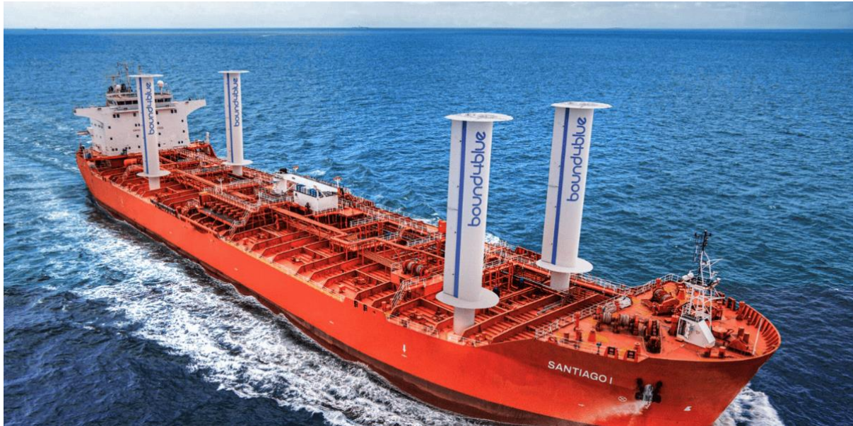
Figure 2: eSAIL system fitted on tanker SANTIAGO I [8]
