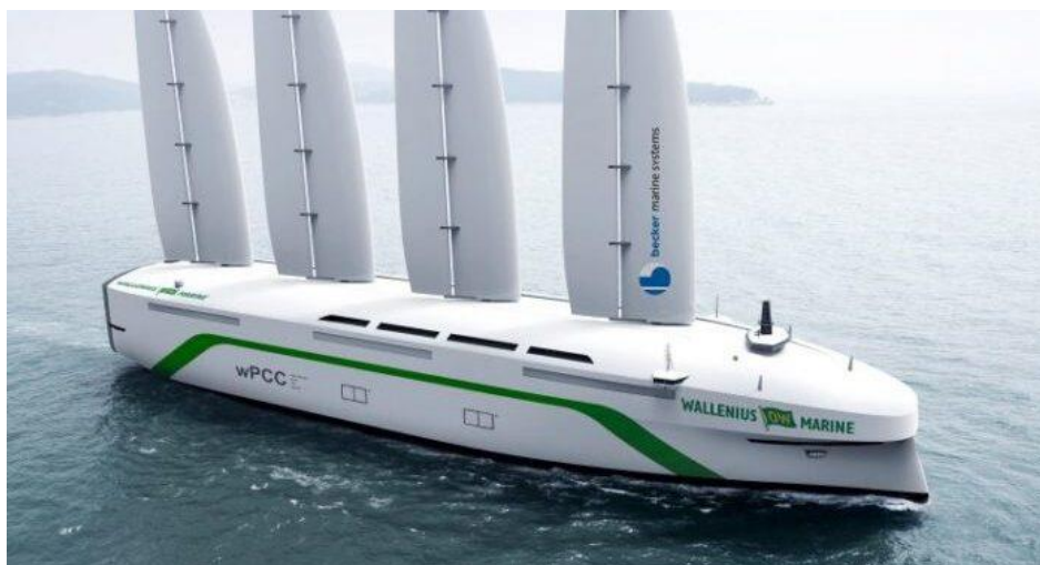
Figure 3: Wing sails on ship [12]
