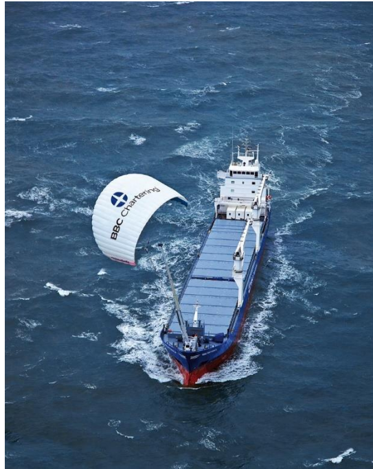
Figure 4: Kite sail on ship [13]
