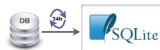
Figure 8.4: Metadata are stored in SQLite tables hosted in DDV server. The update mechanism wakes up once every 24 hours.
