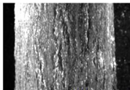
Model Head: 153 m Nozzle opening: 80% Jet diameter: 34mm
