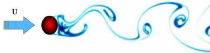
Figure 1-1: Von Kármán vortex street at Re=140 by S. Taneda, Van Dyke (1982).
