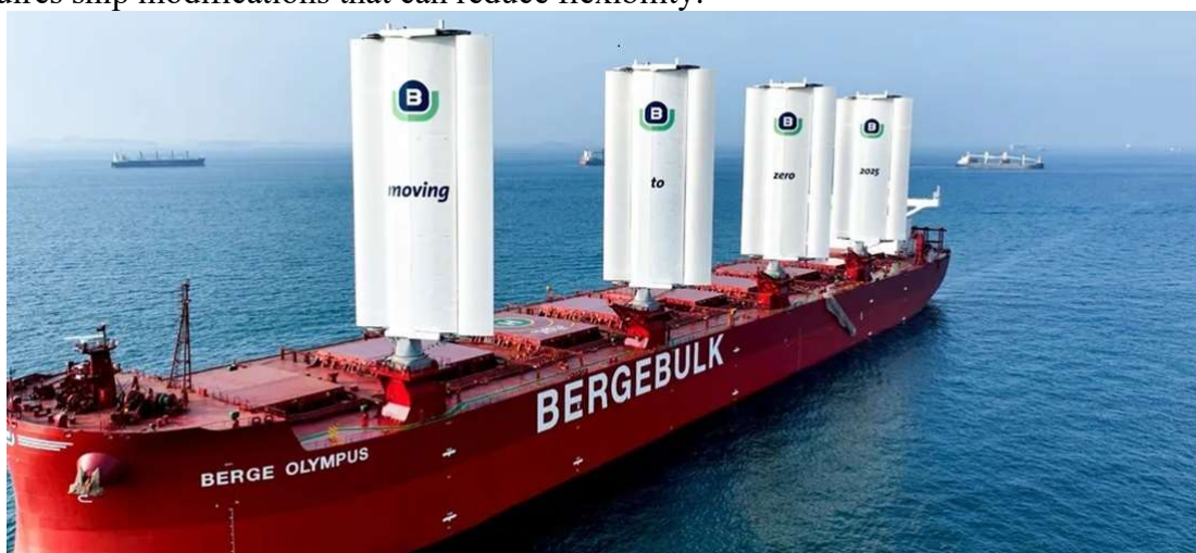
Figure 3: Berge Olympus fitted with four Rigid sails [54]
