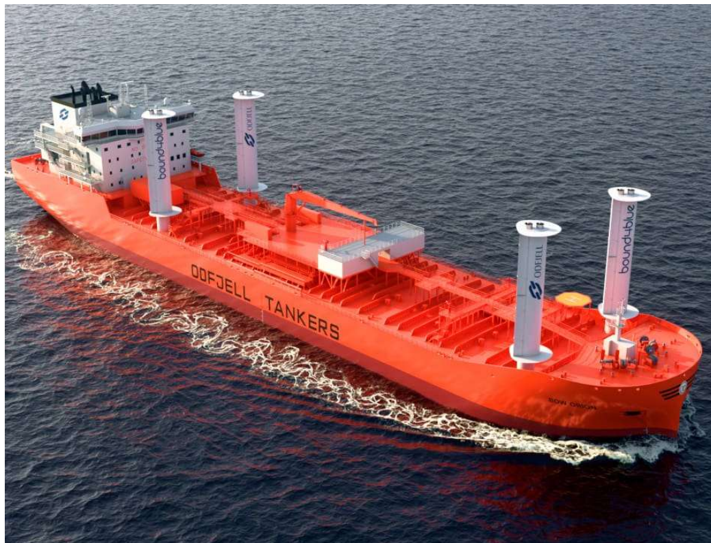
Figure 4: eSAIL system retrofitted in vessel Bow Olympus [56]
