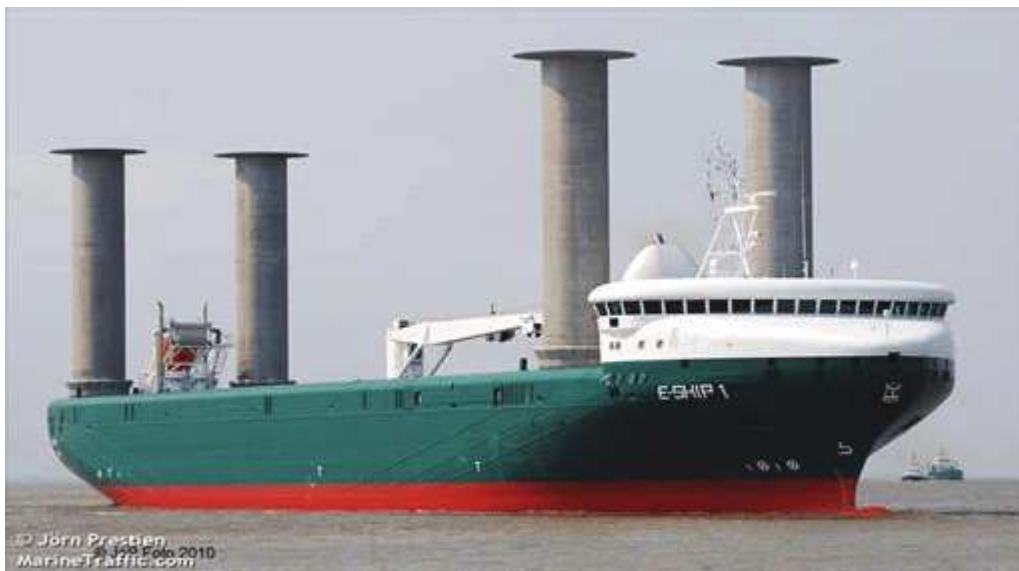
Figure 1: E-Ship 1 equipped with four Flettner rotors [53]
