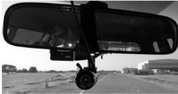
Figure 7. A camera was aimed at the driver to track head position and eye glances
