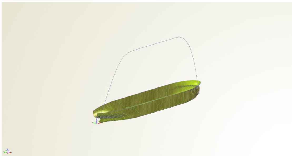
Picture: 3D view of the transformed hull
