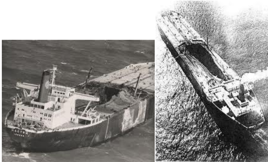
Picture [2]: M/T Mactra after an oil tank explosion. Afterwards Shell introduced tank inerting
