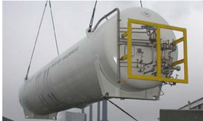
Picture [17]: Example of IMO C-Type tanks used in the Bit Viking Project
