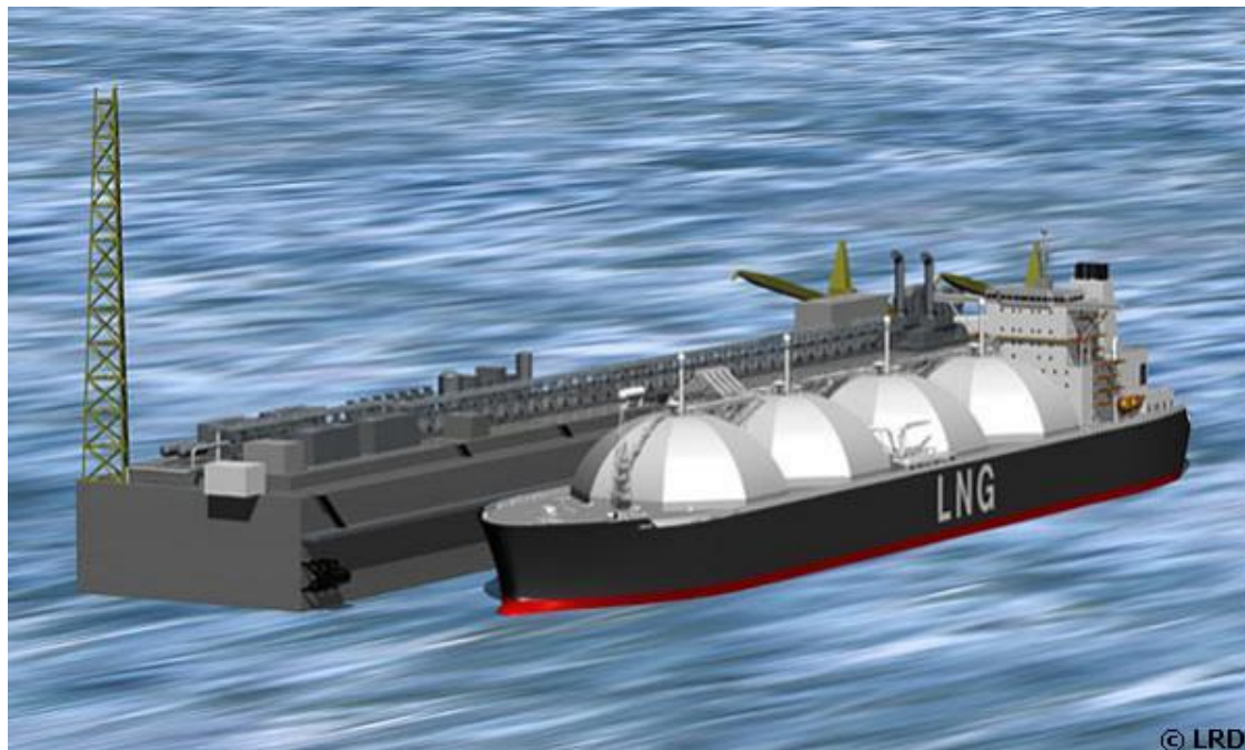
Figure 1-2: LNG-carrier during its procedure of unloading along a FSRU.
