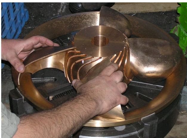
Fig. E.7. Left: Turgo turbine before assembling. Hub slots are visible. Right: Another view of the runner.
