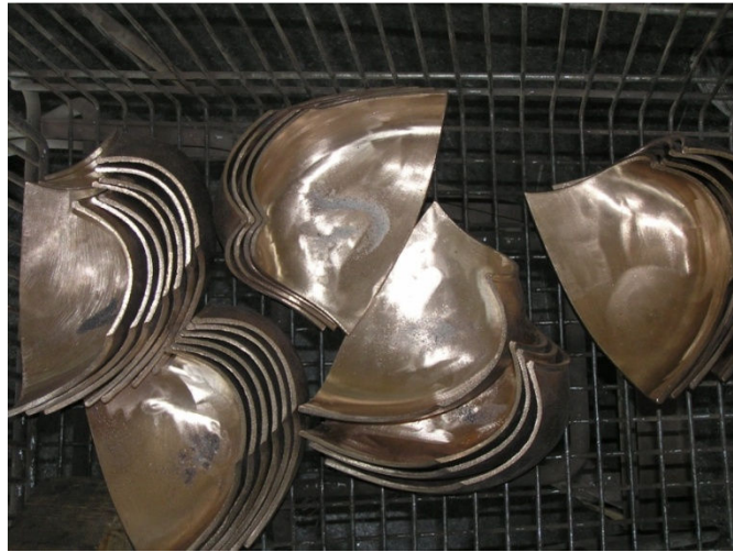
Fig. E.6. Turgo turbine blades after final casting.
