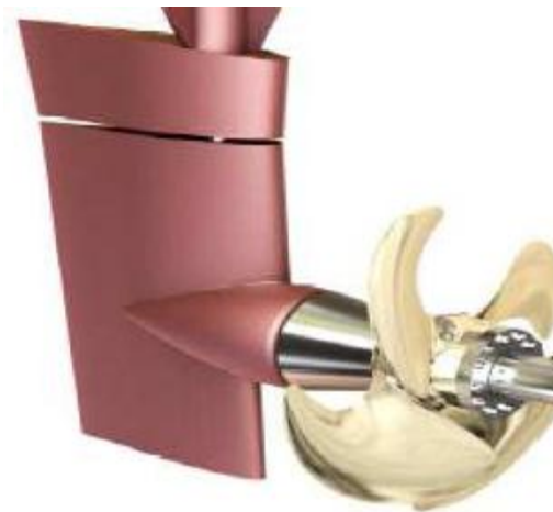
Picture 3.18- Rudder Bulb Hubcap [2].
