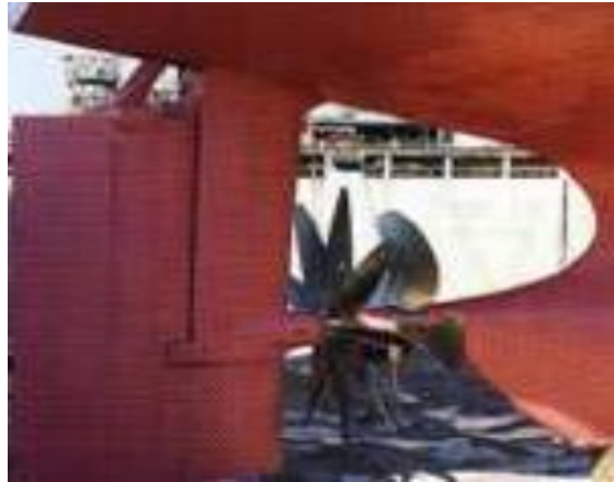
Picture 3.15- Rudder Stator Fin [2].
