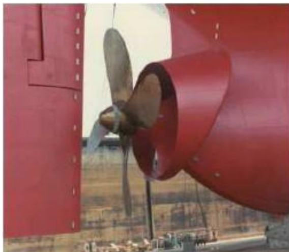
Picture 3.8- Wake Equalizing Duct [2].
