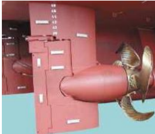
Picture 3.17- Efficiency Rudder [2].
