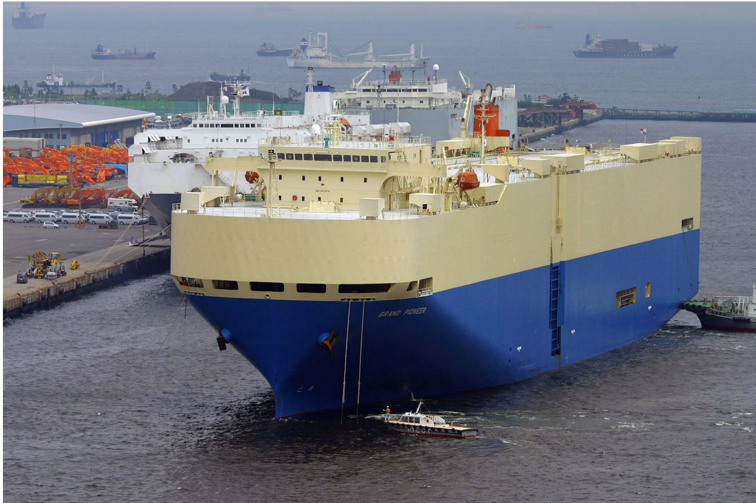
RORO, 1,5 MVA connection 25000 GT
