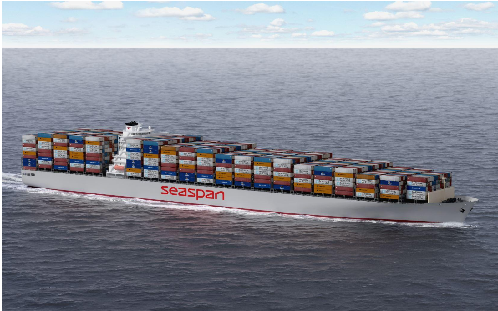
CONTAINER 7 MVA Connection, 7500 GT/6500TEU (500 reefers)
