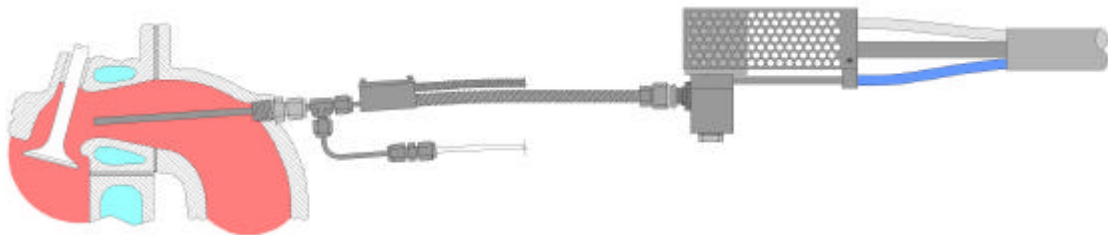
Suitable location of the sampling system in an engine for exhaust port transient NO measurement.
