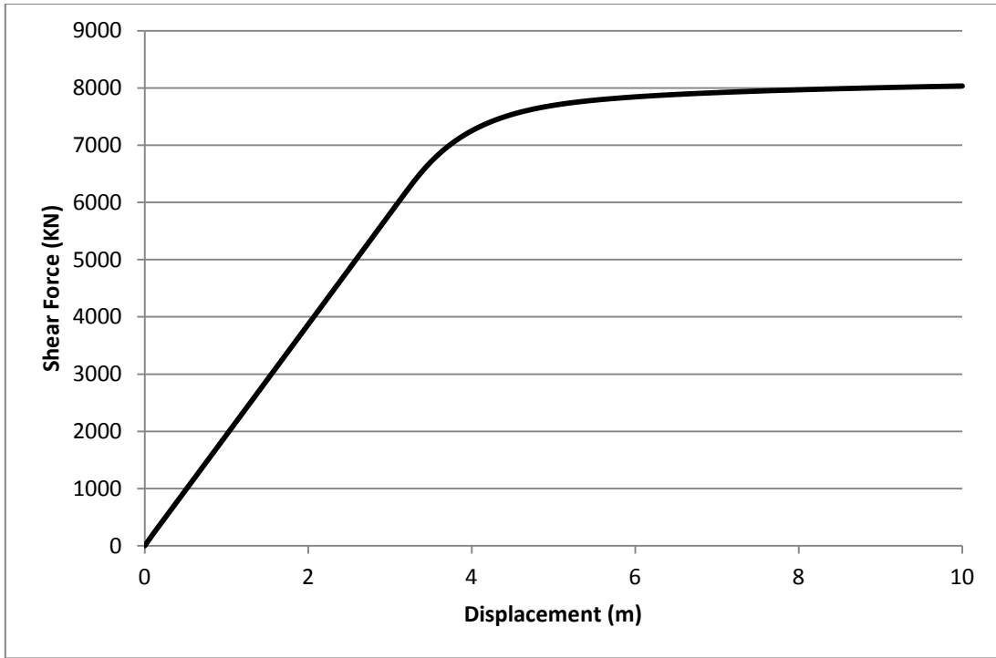
4.5 Capacity curve for tower height H=80 m
