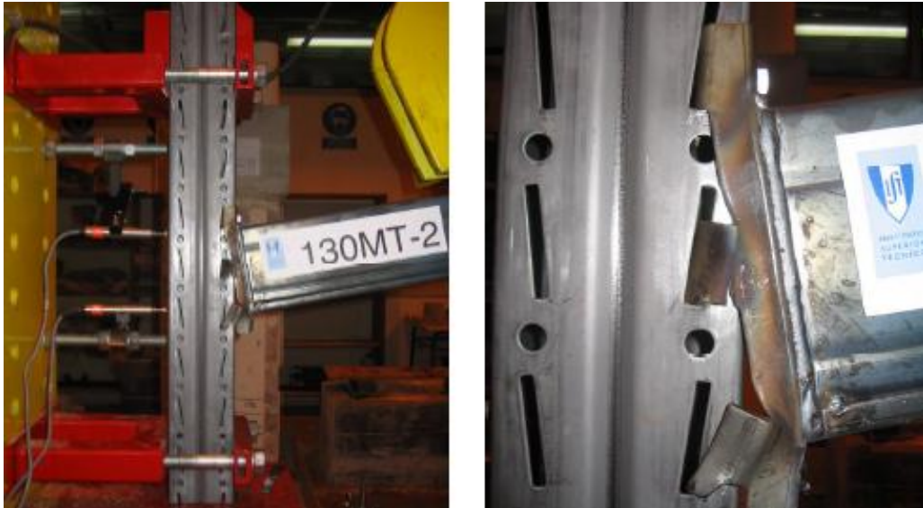
2.4: Typical collapse mode under sagging bending moments
