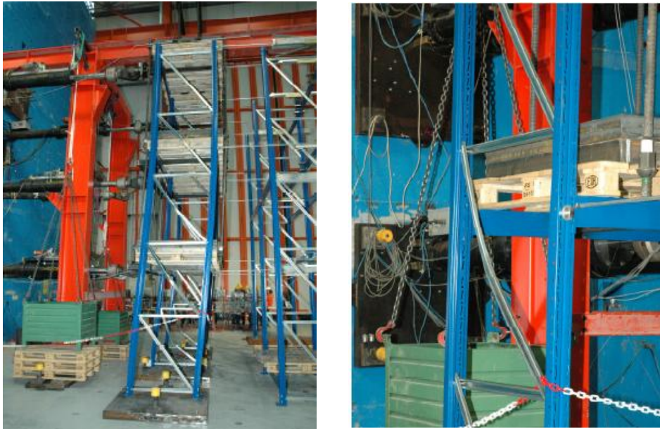
Figure 2.7: Deformed shape and buckling of the diagonals
