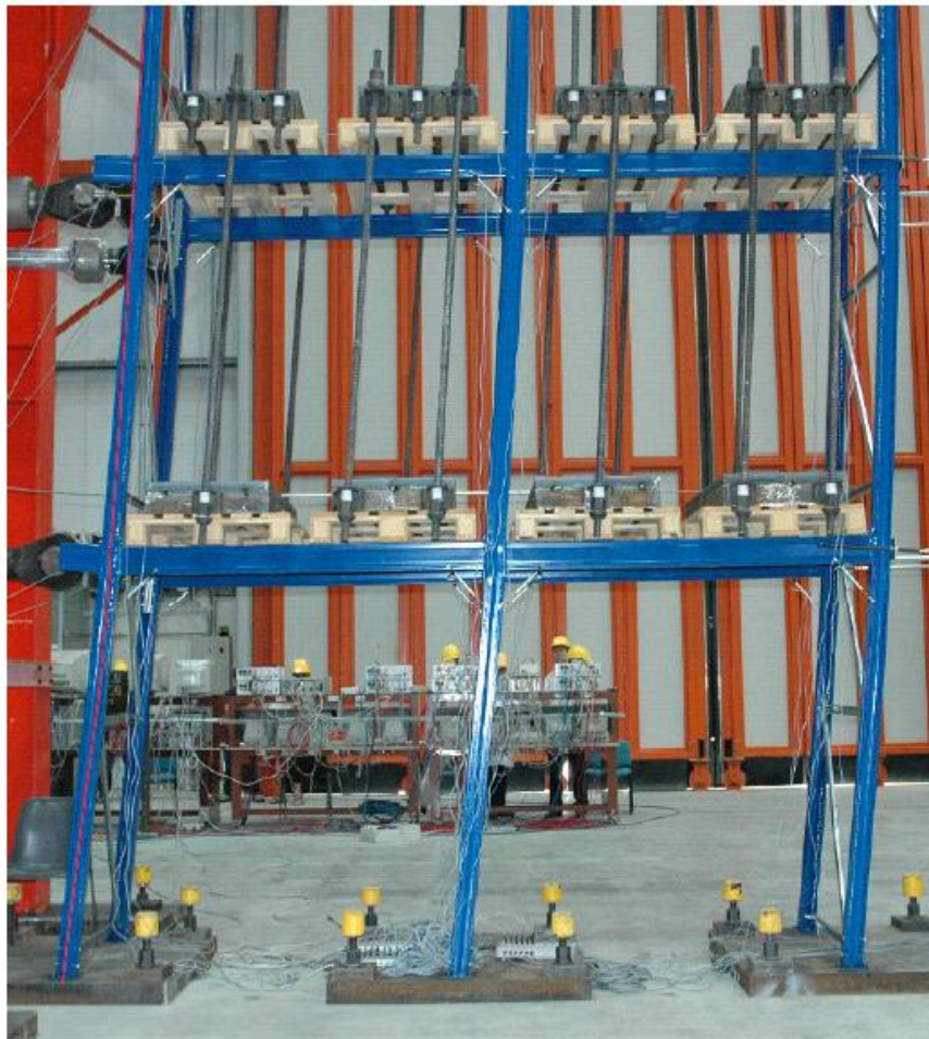
Figure 2.5: “soft-floor” type of collapse mechanism
