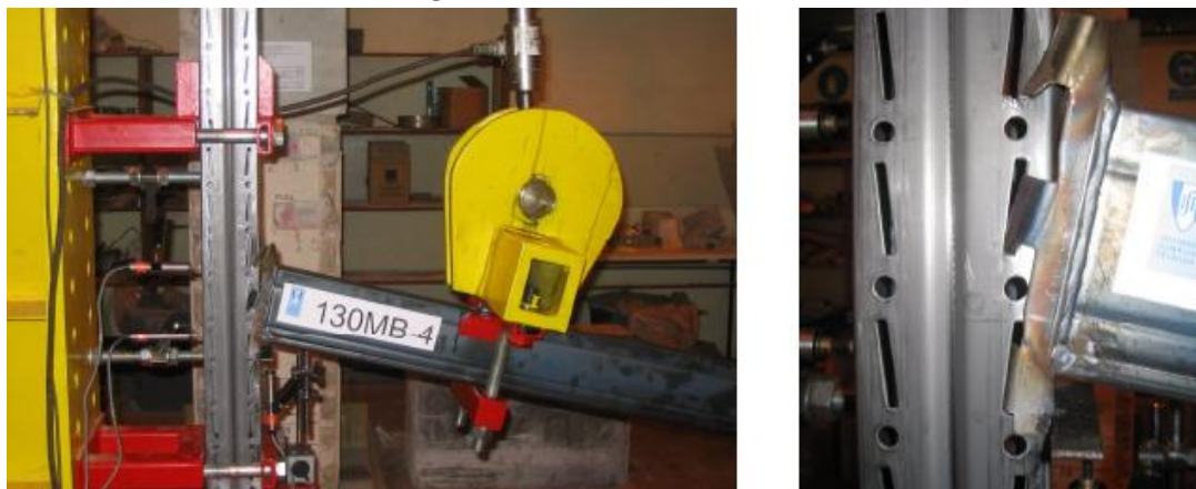
2.3: Typical collapse mode under hogging bending moments
