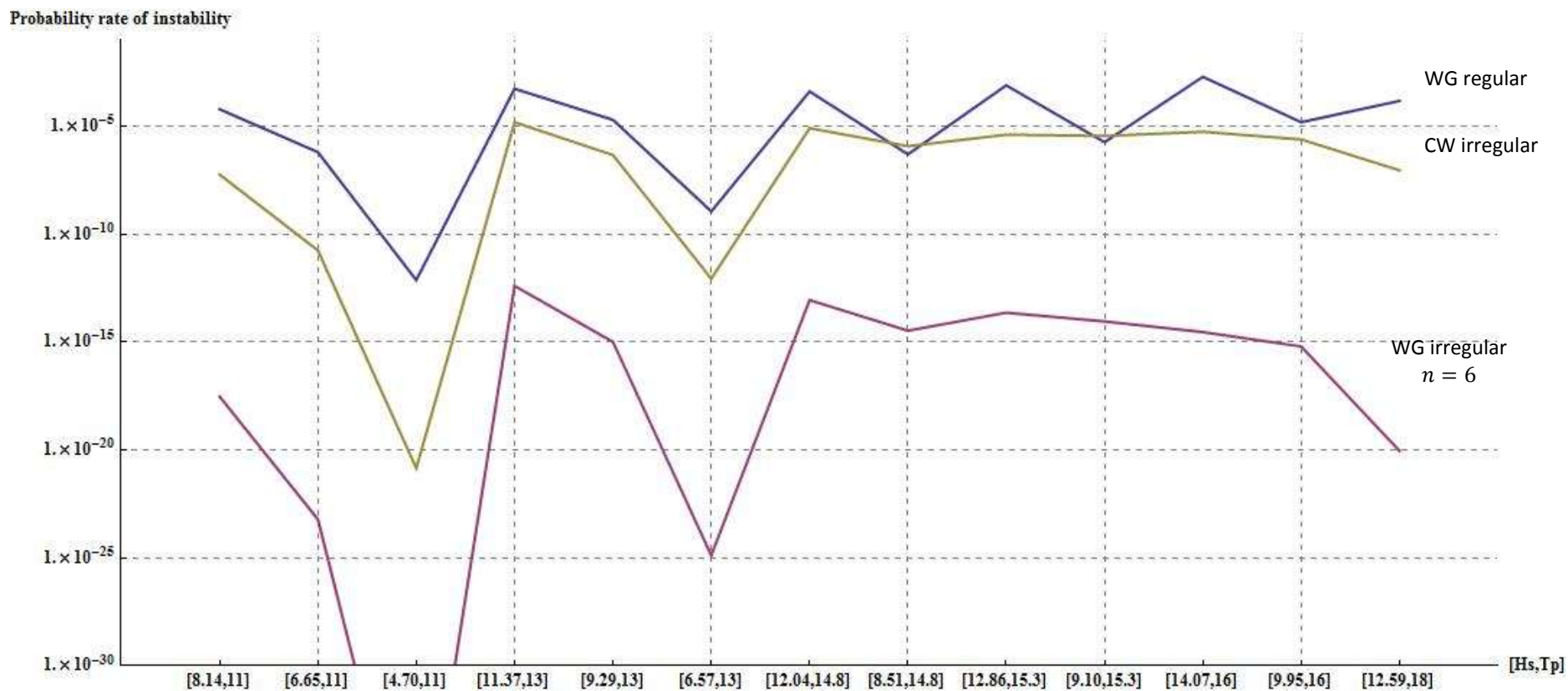
Figure 7.16: Probability rate of capsizing – Comparative diagram (logarithmic scale)
