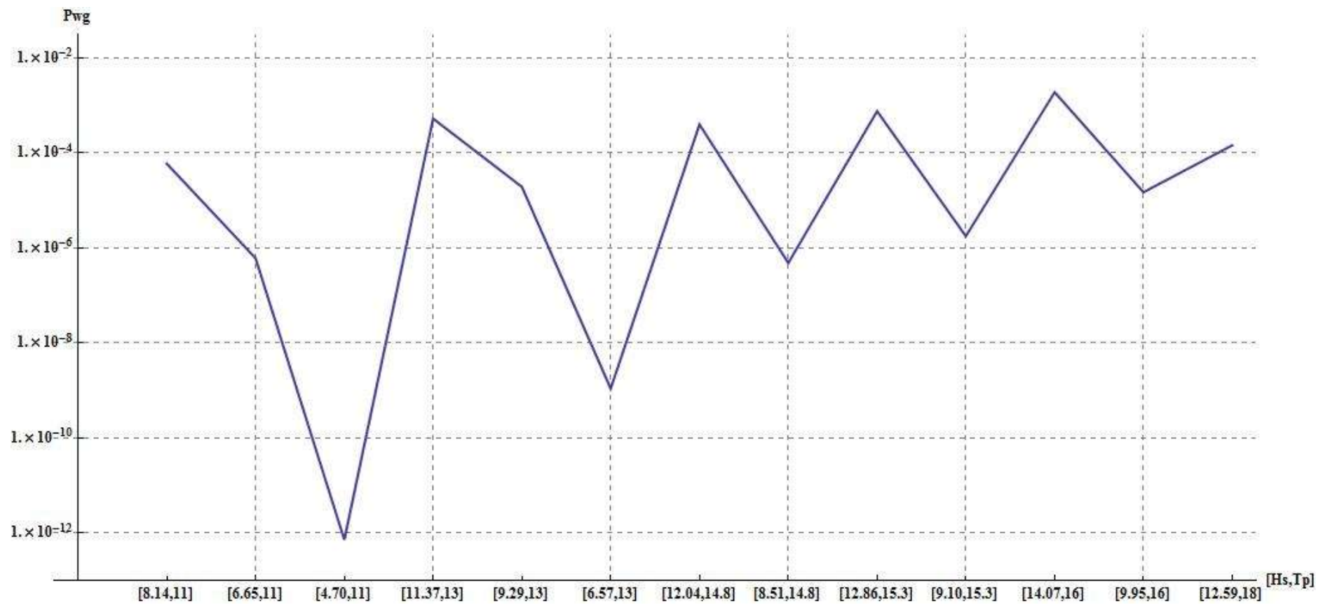
Figure 7.9: Probability rate of capsizing – Wave Group theory on regular waves
