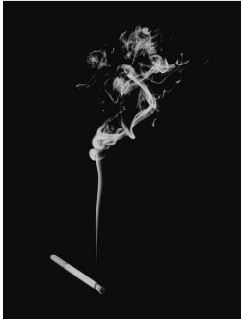
Figure 3. 4: Laminar (below) and turbulent (above) flow of cigarette smoke. The turbulent flow leads to significant increase of mixing of smoke with the ambient air. Source: www.cfd-online.com ( http://i.minus.com/ic1nQ8.jpg )
