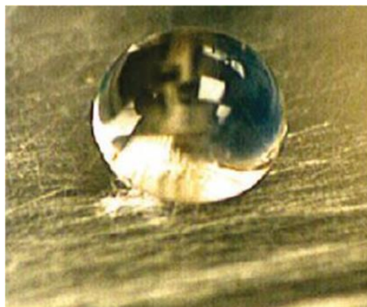
Figure 19 : Superhydrophobic structure with Electrospinning
