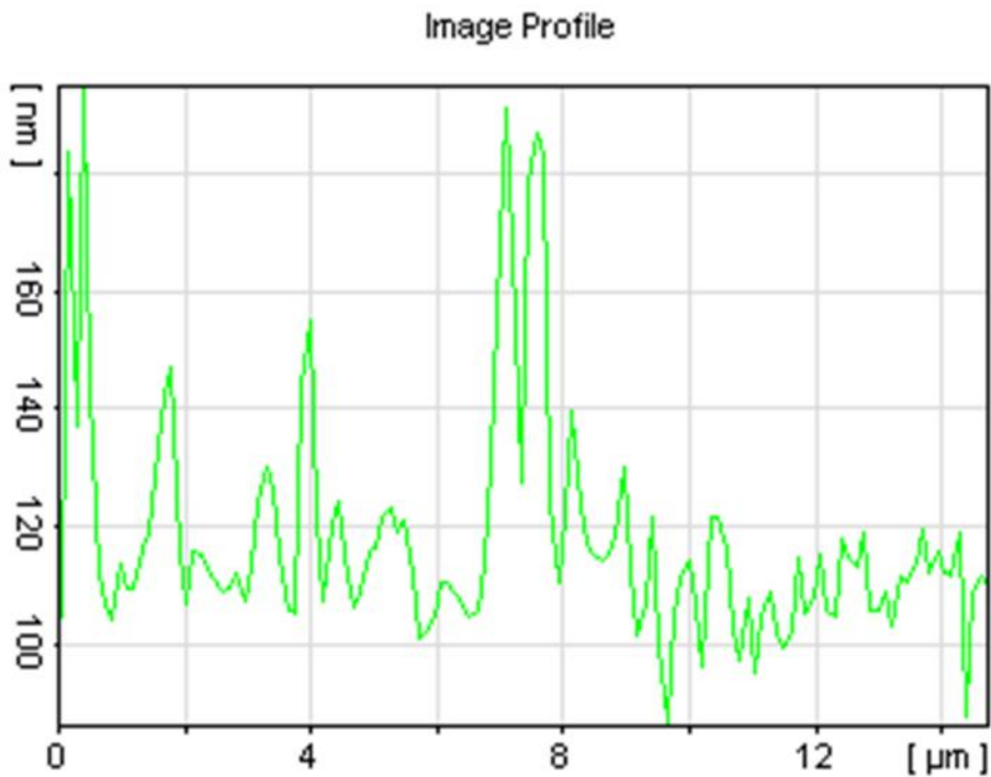
Figure 105 : A cross-section of the Super-hydrophobic film on copper surface
