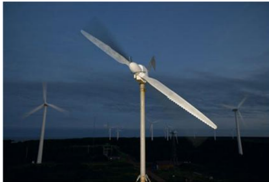
Figure 5 : Whalepower Wind Turbine
