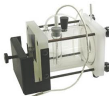
Figure 638 : The three-electrode cell of our lab
