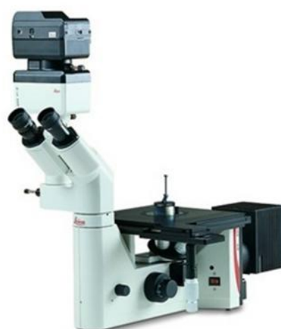
Figure 65 : The inverted metallurgical microscope of our lab Leica DMICM
