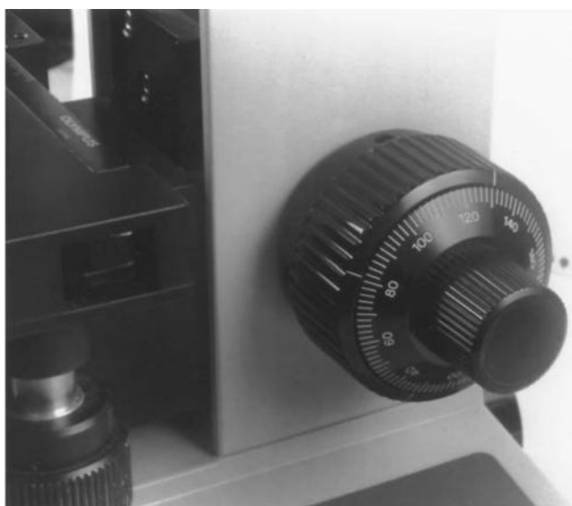
Figure 67 : Coaxial knurled knobs for fine (small, inside knob) and coarse (large knob) focus. Note the graduated scale on the fine-focus knob, which indicates the amount of vertical (z-axis) movement.
