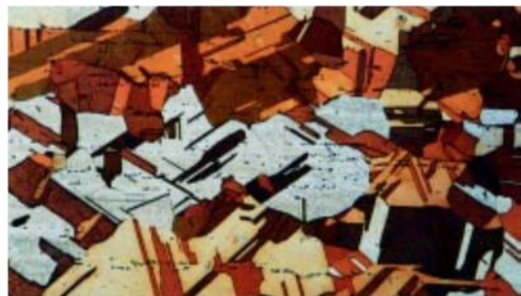
Figure 61: Annealed electrolytic tough-pitch copper prepared by the contemporary method plus a brief vibratory polish (Klemm's II reagent, 50X, crossed-polarized light with light use of sensitive tint.)
