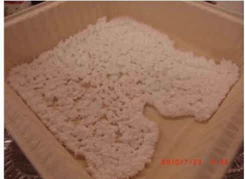
Figure 30 : Aluminum Pan with Super Hydrophobic Coating
