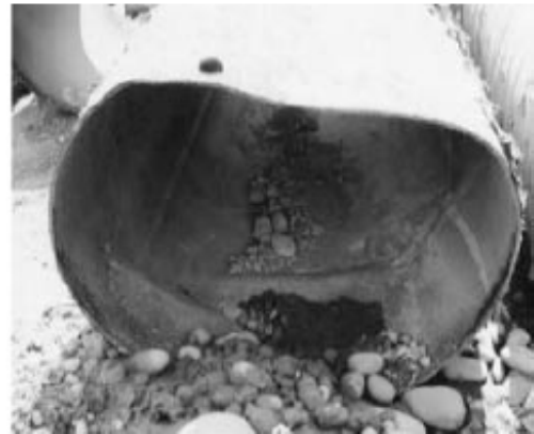
Figure 1.5.8. Large deformation of steel pipe section crossing an active fault (1999 Chi-Chi earthquake, Takada et al.2001).
