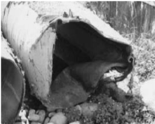
Figure 1.5.8. Large deformation of steel pipe section crossing an active fault (1999 Chi-Chi earthquake, Takada et al.2001).
