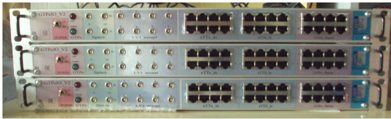
Figure 2.22: Picture of the GTPe modules tested at Demokritos before sending to CERN.
