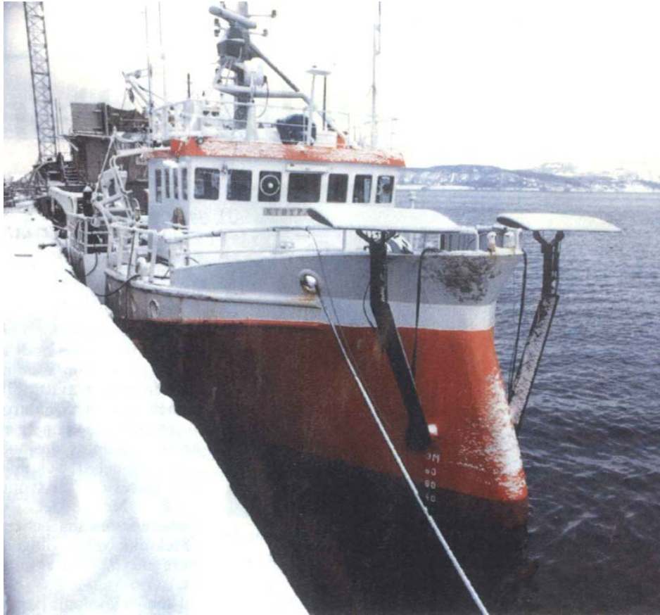
Figure 4: Jakobsen equipped fishing research vessel Kystfangst, owned by the Institute of Fishery Technology Research, with a bulbous bow and two foils on each side of the bow (Dybdahl, 1988).
