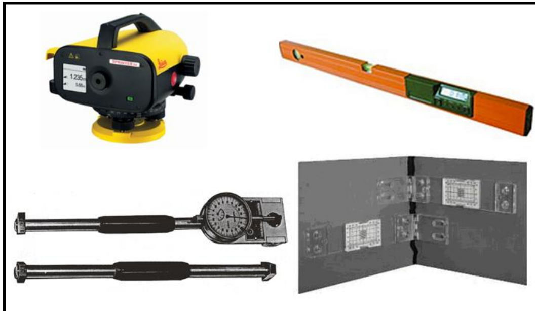
2.1: a) Leica b) Digital inclinometer c) Extensometer and d) 3-direction crackmeter
