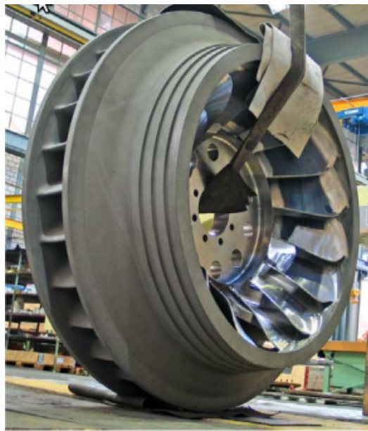
Figure 5.18: Optimization of a Francis Turbine: An existing runner which is quite similar to the one designed herein, is shown, (2).
