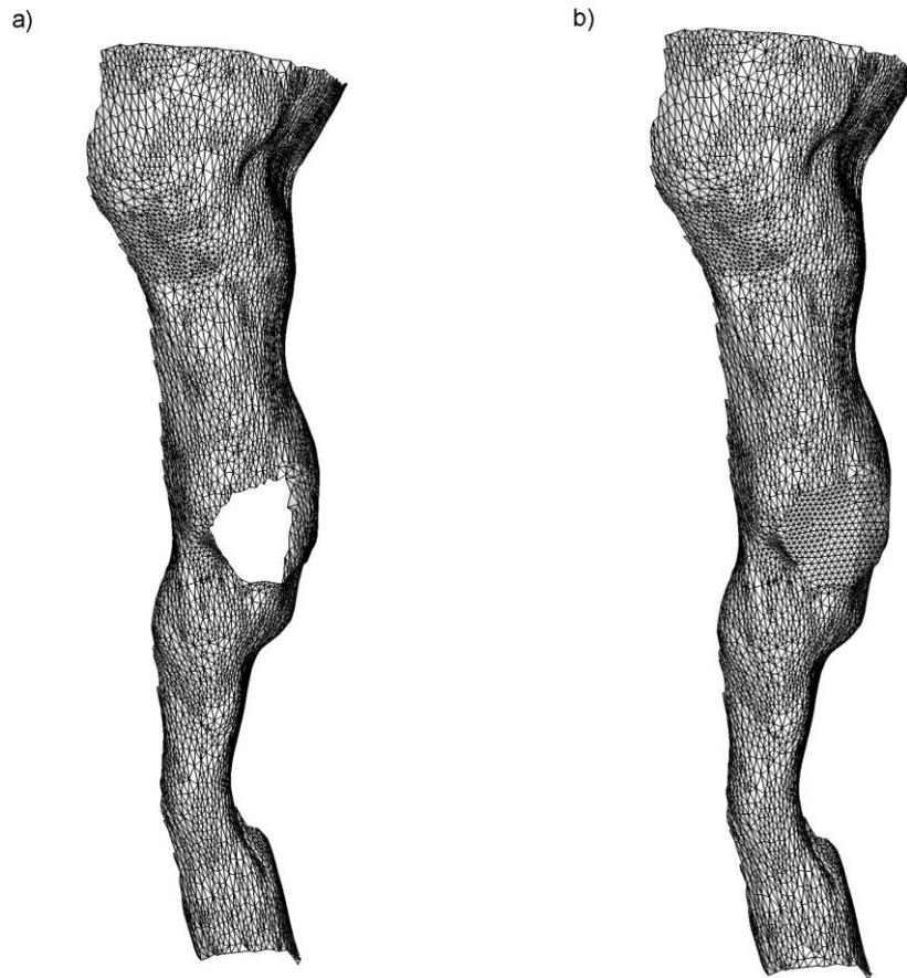
**Figure 3.16: (a) The left manifold that the branch is united. (b) The same manifold with the hole filled with triangles.**
