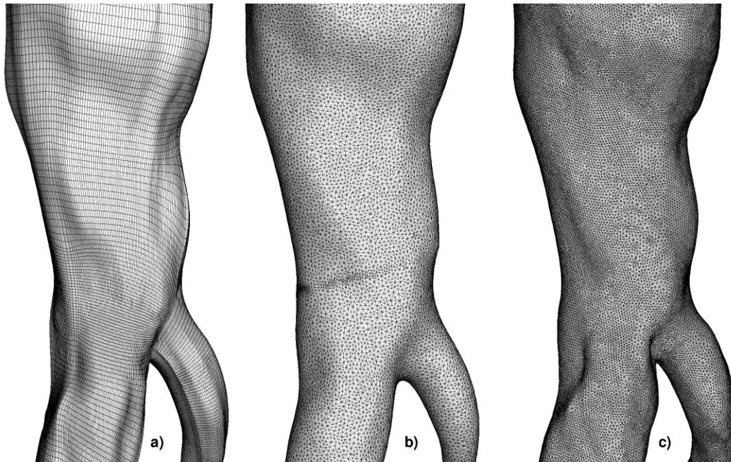
**Figure 3.21: A view of three grids used for the comparison. (a) The structured grid S3 (b) The “coarse” unstructured grid U1. (c) The “fine” unstructured grid U3.**
