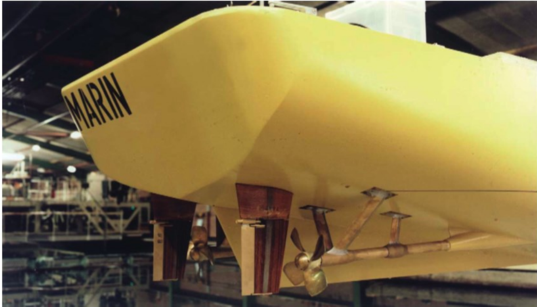
Figure 2. Typical optimised aft ship design of a conventional cruise vessel with twin propeller/twin rudder arrangement
