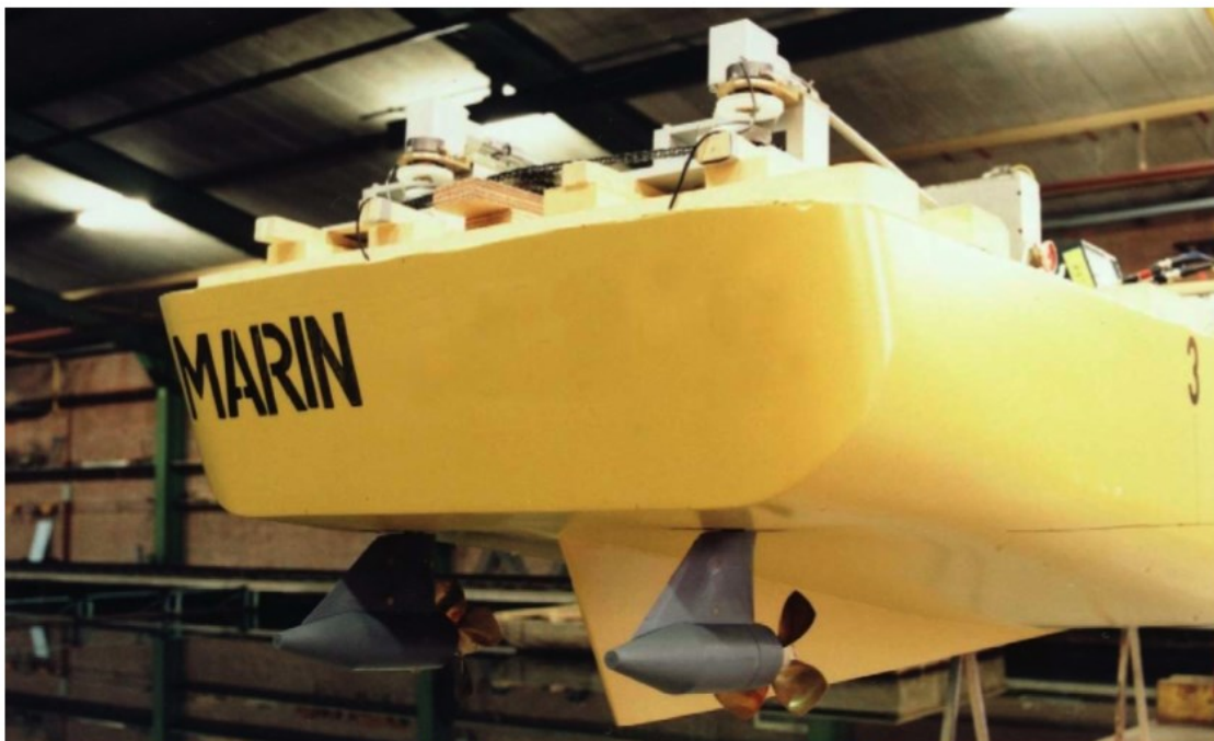
Figure 3. Typical optimised aft ship design of a cruise vessel with podded propulsion and steering arrangement
