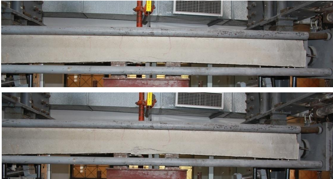
Figure 5.13: Crack pattern of the seventh beam.
