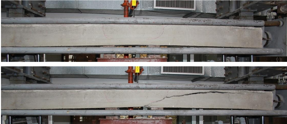
Figure 5.11: Crack pattern of the sixth beam.
