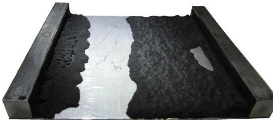
Figure 2.22: Multilayer particle deposits after a flow transient corresponding to a friction velocity u^* = 0.36 m/s, flow direction from left to right (Barth et al., 2013).
