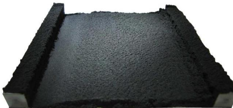
Figure 2.20: Multilayer particle deposits between step 13-14 after t = 4 h, flow direction from left to right (Barth et al., 2013).
