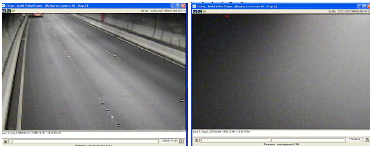
Figure 27: How smoke may render the CCTV useless in only 60 seconds (Dix 2011)
