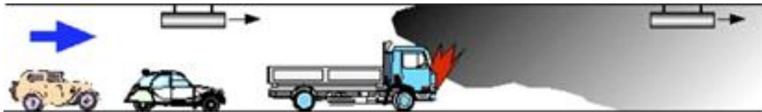
Figure 6: Longitudinal ventilation system
