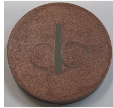
Figure 42 Sample mounted in a copper resin (30mmØ)
