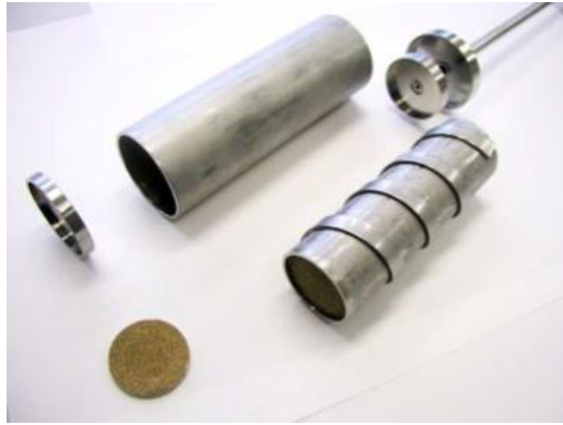
Picture 3.15: The trap used in the gas purging system.
